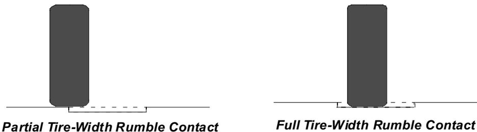
Full tire-width rumble contact allows the tire to fully drop into the rumbles. It is the loudest interval of a rumble strip crossing and is most effective at getting drivers' attention. Its duration *doubles* when rumble width increases from 12" to 16" (assuming an 8" tire contact patch).
